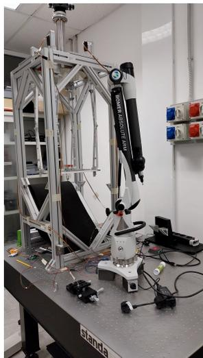
**Figure 1** DORA in action in the deployed configuration in the lab with Romer Hexagon absolute arm standing in front of it.
