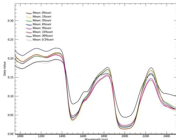
Figure 3. SWIR spectra of different concentrations of Martian simulants.
