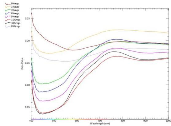
Figure 4. VNIR spectra of different concentrations of Martian simulants.
