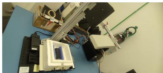
Figure 1. Set-up: hyperspectral camera and its accommodation for acquiring spectra of icy samples.
