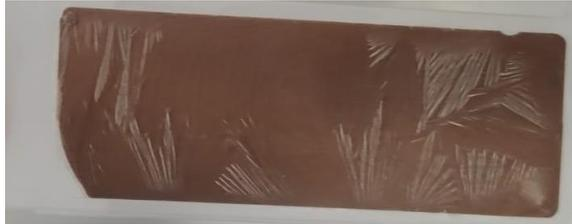
Figure 2. Icy slab of 30% Martian simulant MGS-1 and 70% water ice.
